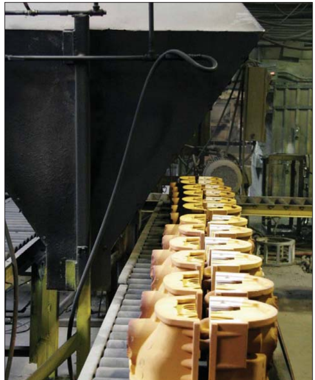
Shell molds ready for assembly and then pouring at the Syracuse, NY, aluminum foundry.
